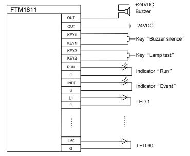
Fig.5 Connection diagram 1
