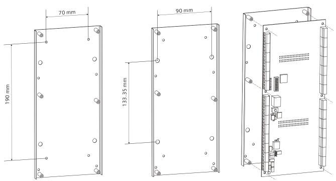
Fig.2 Installation size for wall-mounted
