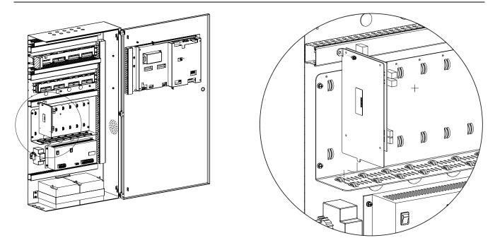
Step1: insert line card into notch on bottom and back plate.
